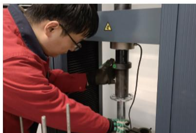
Shear Strength of Welds Check the girth weld on the inner side of Rosettes
