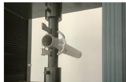
Tensile Strength Test Maximum tensile strength Rosettes can withstand during the stretching process
