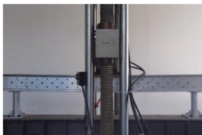
Load Capacity Test Aluminum Beam
