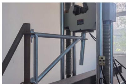
Load Capacity Test Side Bracket
