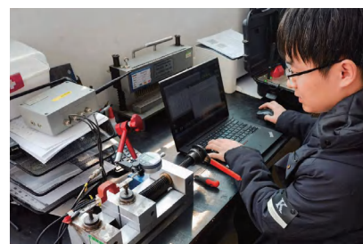
Strain Gauge Accuracy Test Sensors accurately measure the deformation and stress of structures
